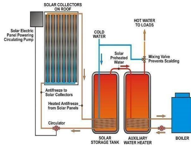
Figure 9 Layout of a conventional solar water heating system [21].
