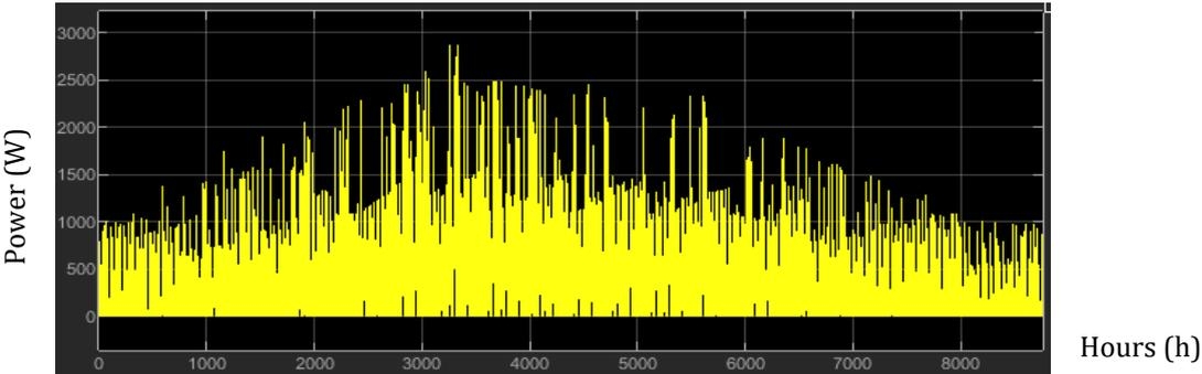
Figure 42 Useful thermal power collected by the solar panels
