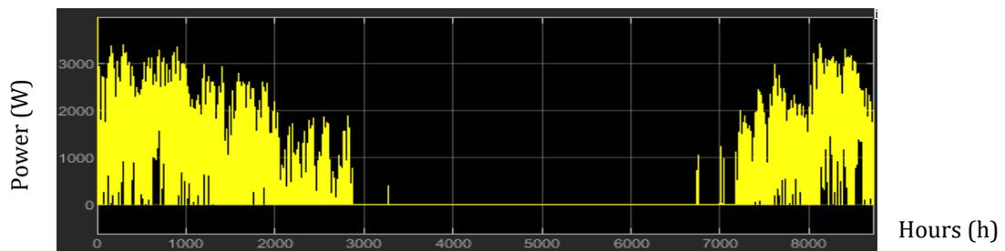
Figure 55 Theoretical back-up power requirements (W)
