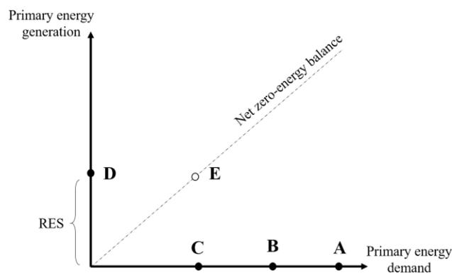
Figure 4 Schematic representation of the nZEB approach [11]
