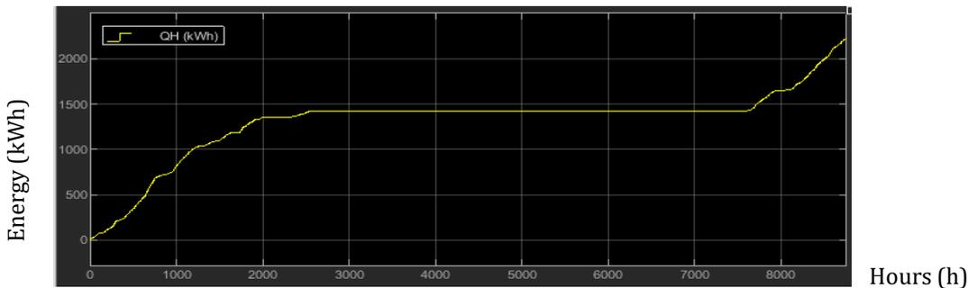
Figure 28 Lisbon's accumulated heating needs (kWh)
