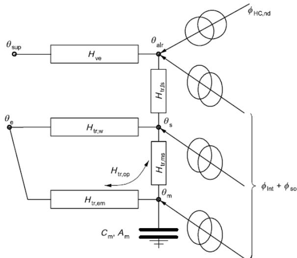
Figure 61 Five resistances, one capacitance (5R1C) model; EN-ISO 13790 standard
