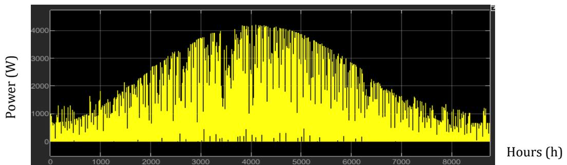
Figure 38 Useful thermal power collected by the solar panels
