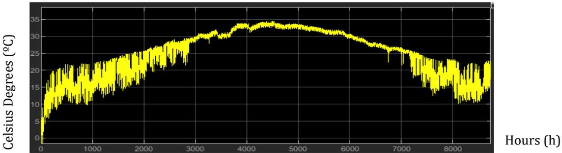
Figure 41 Return temperature to the collector:  $T_{i, coll}$  (°C)
