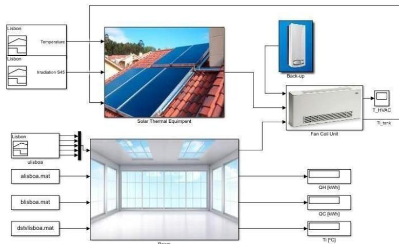
Figure 22 Layout of the complete thermal system model
