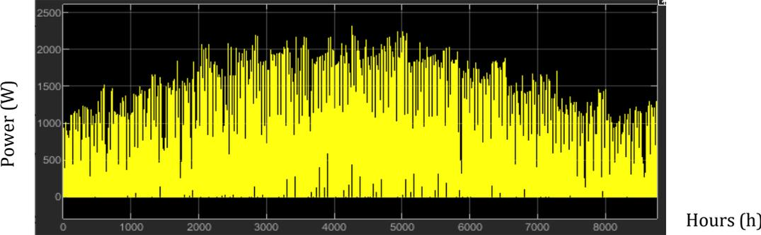
Figure 34 Useful thermal power collected by the solar panels
