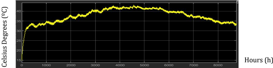
Figure 43 Temperature at the collector outlet:  $T_{u, coll}$  (°C)
