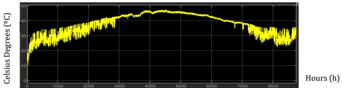
Figure 54 Return temperature to the collector:  $T_{i, coll}$  (°C)
