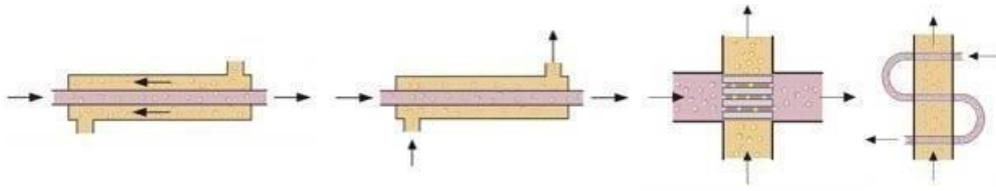
Figure 7 Counter flow, co-current flow, cross flow and cross/counter flow types of HE [18]
