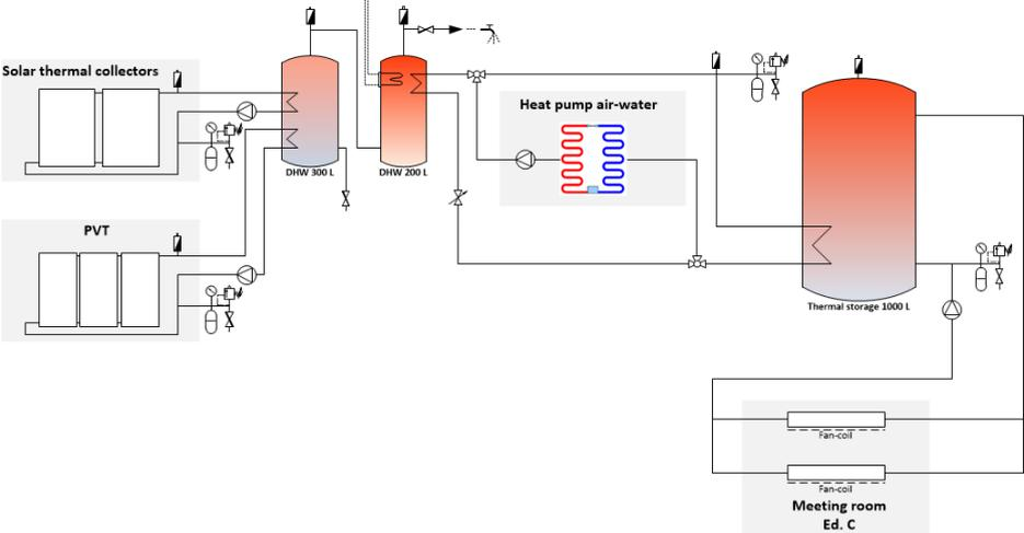
Figure 17 LNEG pilot plant thermal system
