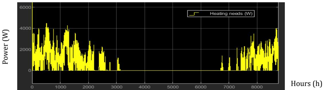
Figure 33 Marseille instantaneous power required for heating purposes
