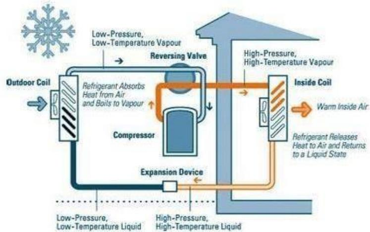
Figure 8 Air source heat pump scheme; Energies [Ref????]
