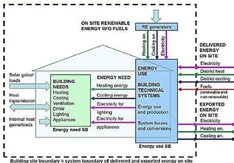
Figure 6 System boundaries for on site assessment and energy flow calculation [14]
