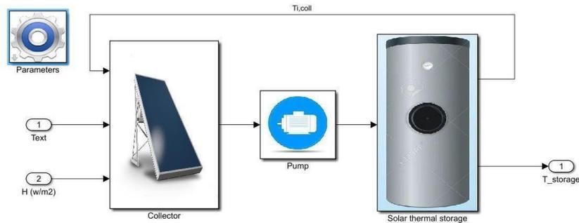
Figure 25 Layout of the Solar thermal sub-system
