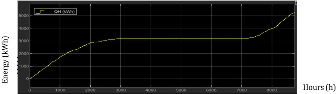
Figure 30 Madrid's accumulated heating needs (kWh)
