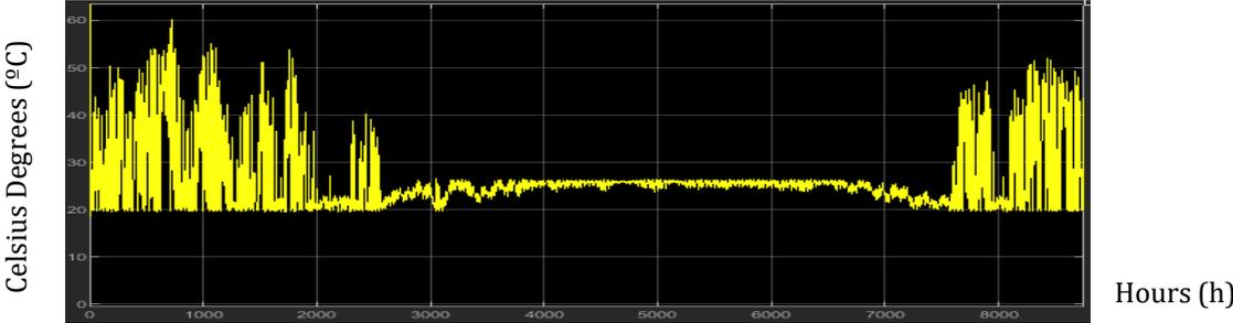
Figure 47 Required HVAC Temperature (°C) in Lisbon
